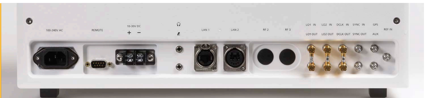
FIGURE 3: EXTERNAL INTERFACES FOR POWER SUPPLY, LAN, GPS ANTENNA AND SYNCHRONIZATION
