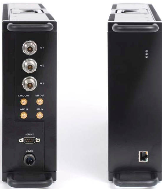
FIGURE 3: EXTERNAL IZT R3410 INTERFACES FOR RF CONNECTORS, SYNCHRONIZATION, SERVICE, POWER SUPPLY AND ETHERNET
