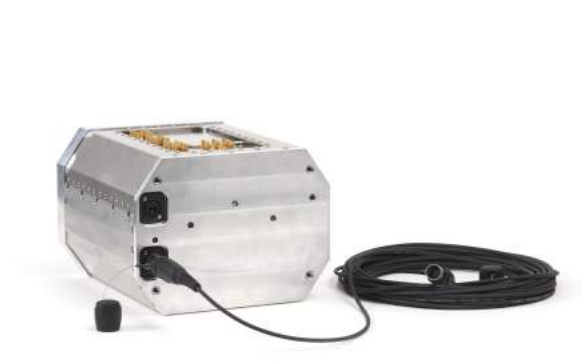
Figure 5: IZT R5506 electronics with hybrid cable
