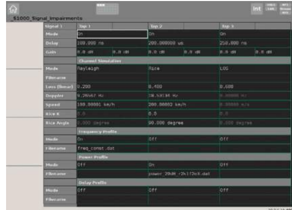
Figure 6: SCREENSHOT OF FADING CHANNEL SIMULATION
